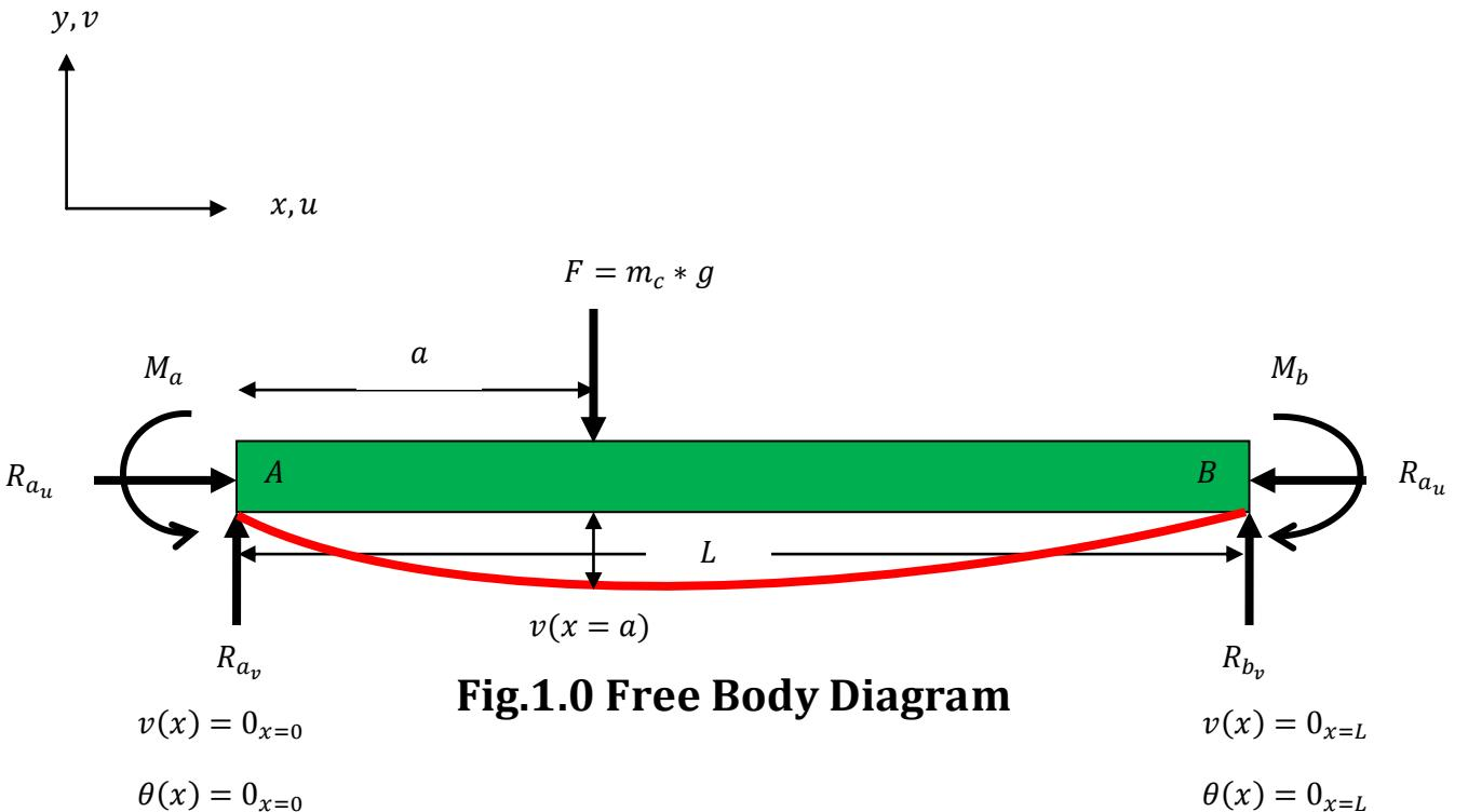
There are six unknowns,  $R_{a_v}, R_{a_u}, R_{b_u}, R_{b_v}, M_a, M_b$ , while only three equilibrium equations are available.
