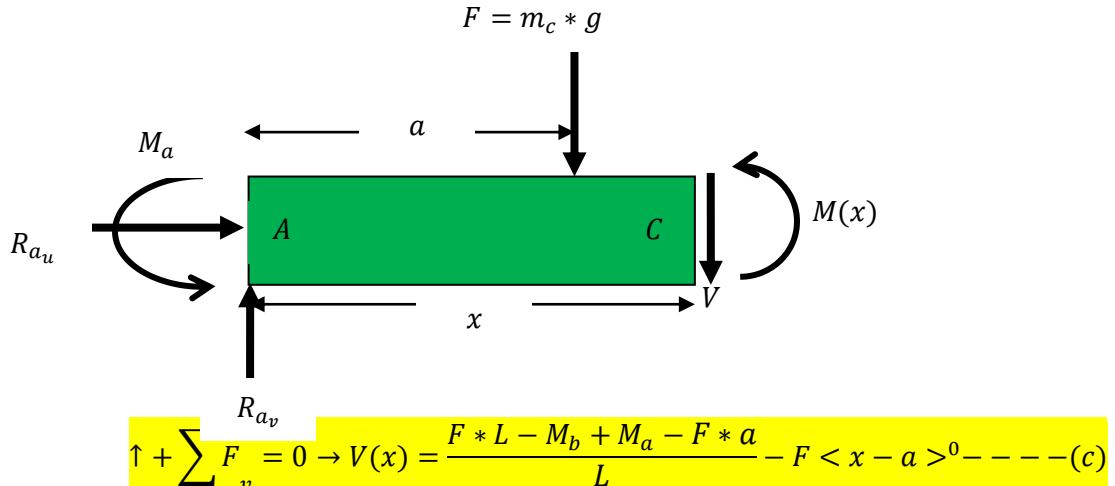
$$\text{anticlockwise(+)} \sum M_c = 0 \rightarrow M(x) = \frac{F * L - M_b + M_a - F * a}{L} * x - F < x - a >^1 - M_a$$
